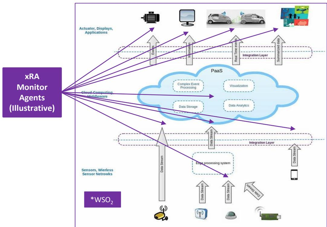
xRA monitoring agents (xRA replicas) may be placed throughout a complex cloud/edge system to extend system observability, enabling operations personnel to compare the performance of various parts of the system.
