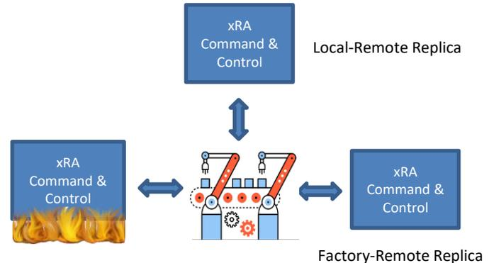
To protect against a controller failure, xRA spatially distributes command and control of the complex algorithms that tie together mission- or life-critical sensors and actuators while retaining the state of the control system
